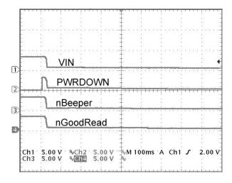
Figure 18. VIN Removed (USB)
